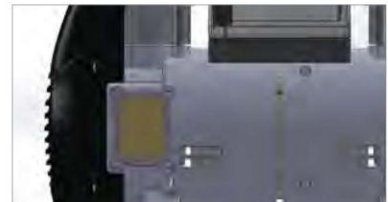
Air In-take Filter (100% wool blanket material)
