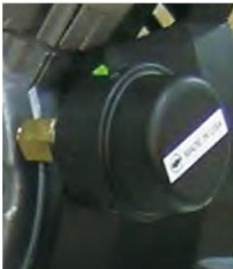
Air In-take Filter (Polyester material)
